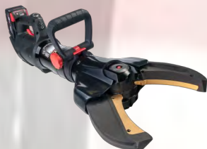
E Force C236 Cutter 7.9" Blade Opening 10,500 psi 236,000lbs Max Cutting Force
