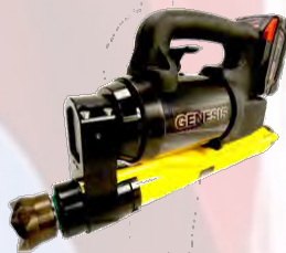
E Force 21/36 Ram 35.8" Opened Lengthed 10,500 psi 24,953lbs Max Spreading Force
